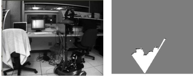
Figure 2: Camera image (left), Occupancy map representing bird's-eye view of obstacles (right)
