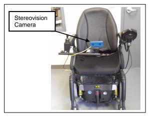
Figure 1: IWS mounted on a Pride<sup>®</sup> Mobility Q6000z Powered Wheelchair.
