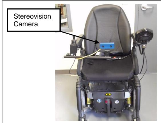
Figure 1: IWS mounted on a Pride® Mobility Q6000z Powered Wheelchair.
